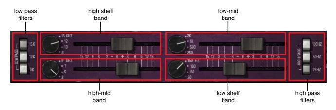
Figure 151. Trident A-Range band control layout
