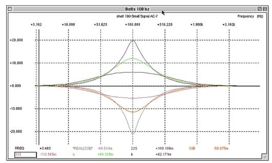
Figure 68. Effect of Bandwidth control on response curve in Bell mode
