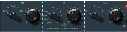
Figure 119. Control grouping within the Pultec MEQ-5
