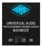
The Power switch determines whether the plug-in is active. This is useful for comparing the processed settings to the original signal or bypassing the plug-in to reduce the UAD DSP load (load is not reduced if UAD-2 DSP Load-Lock is enabled).
