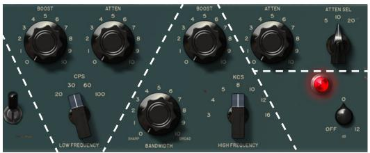
Figure 118. Control grouping within the Pultec EQP-1A
