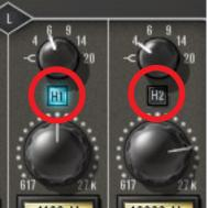
Each band can be individually engaged with the Enable button. All bands default to disabled. When a band is enabled, the button glows blue. To enable a band, click the Enable button or move the band Gain knob.
