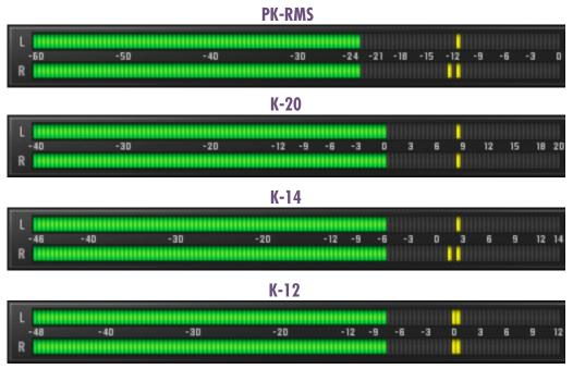
Figure 109. Precision Limiter Meter Types
