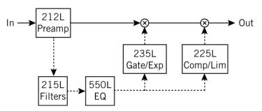
Figure 13. Signal flow with SC enabled in both 215L and 550L modules
