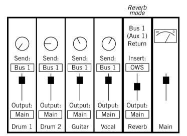
Figure 93. DAW signal routing in Reverb mode using a traditional effect send/return configuration.
