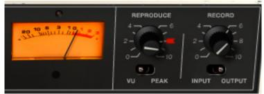
Figure 3. One side of the Ampex ATR-102 "penthouse" showing meter and I/O controls
