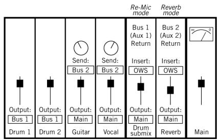
Figure 95. DAW signal routing in a workflow with two Ocean Way Studios plug-in instances. One uses Re-Mic mode for the drum submix, and the other uses Reverb mode for the guitar and vocals.
