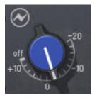
The Input Gain control sets the level at the input of the plugin, and doubles as a plug-in bypass control. The range is from -20 dB to +10 dB, and off.
