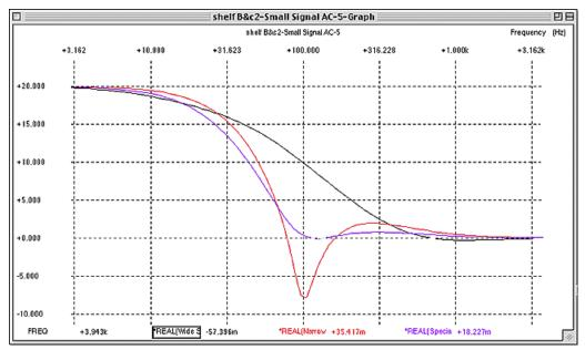
Figure 69. Effect of Bandwidth control on response curve in Shelf mode
