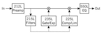
Figure 9. Signal flow with 215L Sweep Filters SC enabled
