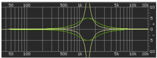
Figure 21. Parametric Type III response
