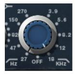
The independent low and high cut filters are controlled by the dual-concentric knobs to the right of the low band (see Figure 77 on page 249). The controls specify the fixed frequency of the cut filter. The cut filters have an 18 dB per octave slope.
