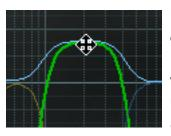
If the cursor is moved slightly lower than the above example, the gain and center frequency can be adjusted simultaneously, without adjusting the bandwidth. In this case the cursor changes to an up/down/left/right arrow when hovered over the hot spot to indicate the direction available for dragging.
