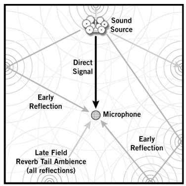
Figure 91. The main signal components in an acoustically recorded sound
