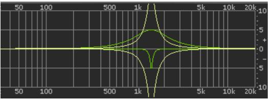
Figure 20. Parametric Type II response
