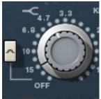
The high band delivers smooth high frequency shelving or peak equalization. The inner knob controls the band gain, and the outer ring selects the frequency or band disable.
