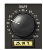
The Shape knob is the primary saturation control for the Maximizer effect. It contours the harmonic content and apparent dynamic range of the processor by changing the small-signal gain of the saturator. The available range is 0-100%.
