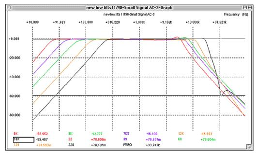
Figure 70. High Pass and Low Pass filter response curves (standard version)
