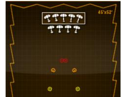
source; conversely, the room gets "bigger" when the mics are farther away from the source. The Ocean Way Studios modeling includes the proximity gain that occurs in the physical realm; the signal can be notably louder as microphones are positioned closer to the source.
