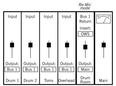
Figure 94. DAW signal routing with OWS in Re-Mic mode on a drum submix
