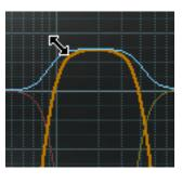
If the cursor is moved to the upper-left region of the three center bands (LMF, MF, HMF), the gain and bandwidth can be adjusted simultaneously, without changing the center frequency. In this case the cursor changes to a diagonal arrow when hovered over the hot spot to indicate the direction available for dragging.
