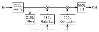
Figure 8. Simplified signal flow illustrating parallel side chain inputs with 215L SC enabled
