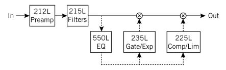
Figure 12. Signal flow with 550L SC enabled
