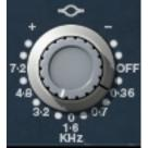
The midrange band is controlled by dual-concentric knobs, delivering smooth semi-parametric midrange equalization.
