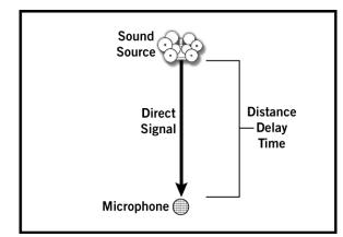
Figure 92. Illustration of Distance Delay. When set to aligned, this "extra" time is eliminated.
