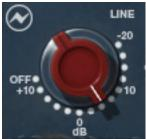
The Input Gain control sets the level at the input of the plug-in. The range is from -20 dB to +10 dB.
