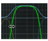
If the cursor is moved to where two bands crossover, the crossover frequencies can be adjusted, without changing the gain or center frequency. In this case the cursor changes to a left/right arrow when hovered over the hot spot to indicate the direction available for dragging.
