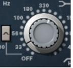
The low band delivers smooth low frequency shelving or peak equalization. The inner knob controls the band gain, and the outer ring selects the frequency or band disable.
