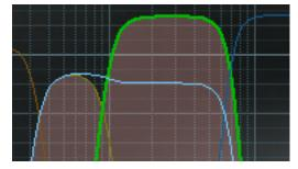
When a band is in Solo mode, its curve in the EQ Display is highlighted.
