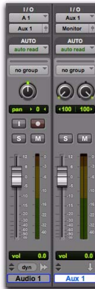
New Auxiliary Input track with audio track output automatically assigned to Bus 1-2
