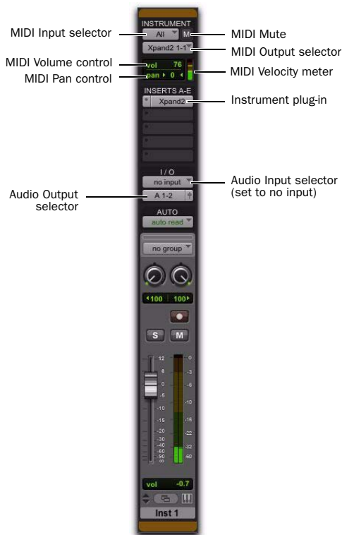
Instrument track configured to control and monitor an instrument plug-in (Xpand 2 shown)
